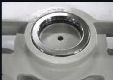
Ball bearing on swinging of saw arm for smooth and steady cutting action.
