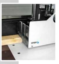
A vertical tail clamp fitted on the pusher, allows for feeding speeds of 240 m/min. while ensuring very precise cutting tolerances of +/- 0.15 mm.
