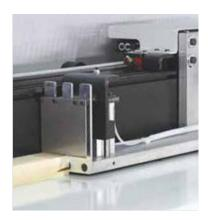
A vertical tail clamp fitted on the pusher, allows for feeding speeds of 120 m/min. while ensuring very precise cutting tolerances of +/- 0.15 mm.
