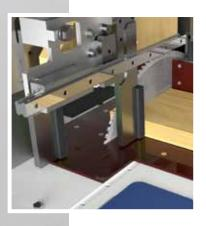
Detail of the cutting area with "Intelligent" front and vertical clamps, riding on high precision linear bearings. The see-through polycarbonate guard, allows for a clear line of sight to the area of the operation of the saw and easy access to the compartment for maintenance, through the assisted lifting of the guard.
